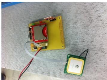
Mounted SD card, pressure sensor and GPS
